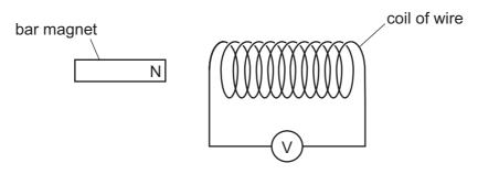
The N-pole of the magnet is moved quickly towards the coil. The voltmeter shows a reading of  $+10 \, \text{mV}$ .
